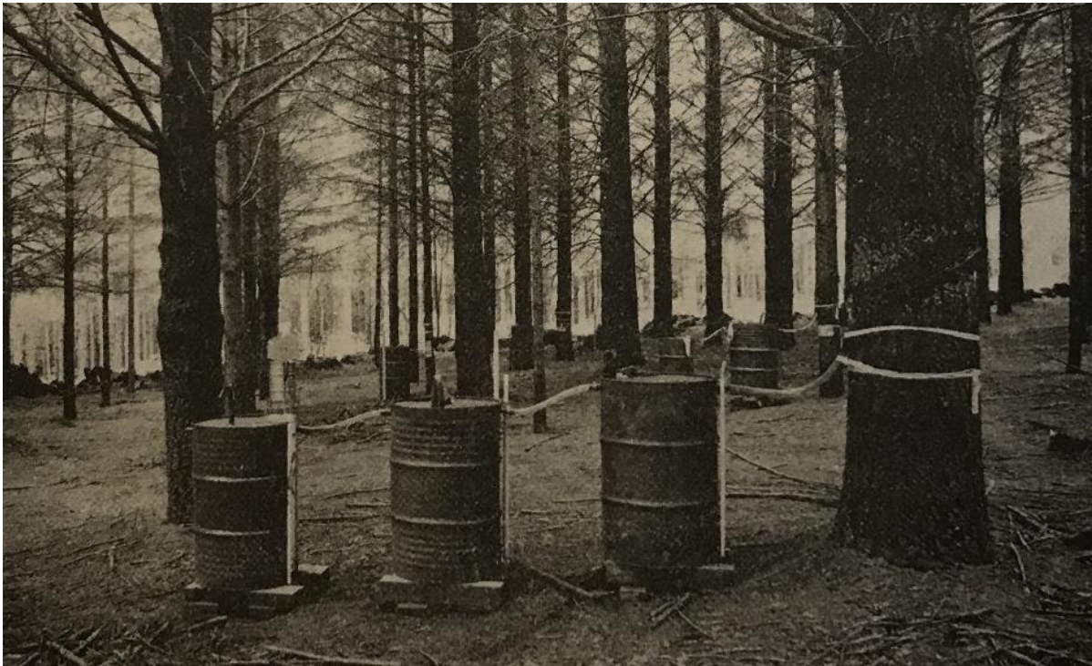
Figure 6. Pared catchment studies undertaken with Douglas Fir species at Cement Creek Plantation, c.1960s-70s. Source: Langford, K. J, and O'Shaughnessy, P. J. 1977. A Study of Canopy Interception in Native Forests and Conifer Plantations . Melbourne: Melbourne Metropolitan Board of Works.
